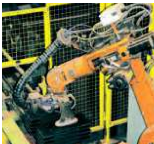
Optimal cable guidance even under extreme conditions, such as here in the Jungmeier roof tile plant
